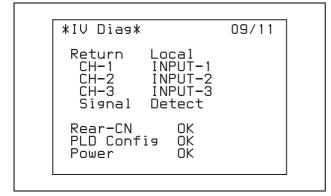
**Return:** Setting status of the return signal input connectors to the return channels from 1 to 3
